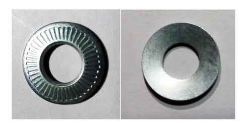
We are manufacturing Conical Contact Washer also known as Rib Washer Single Side Serrated Washer as per STD NFE 25-511 and customer requirement. This washer are conical shaped formed with plane mounting side and top serrated side. The serrated side of the washer exerts circular locking force at the internal face of the bolt head or nut. The top serrated side increases locking force and prevent the loosening of bolt during vibration & pressure.
