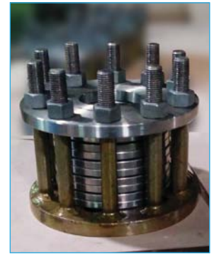
Disc Springs Stack used in Transformer
