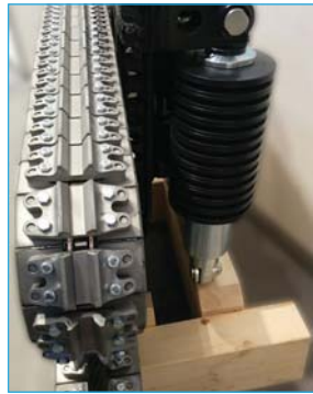
Disc Springs Used in Cable Rope Way Brakes
