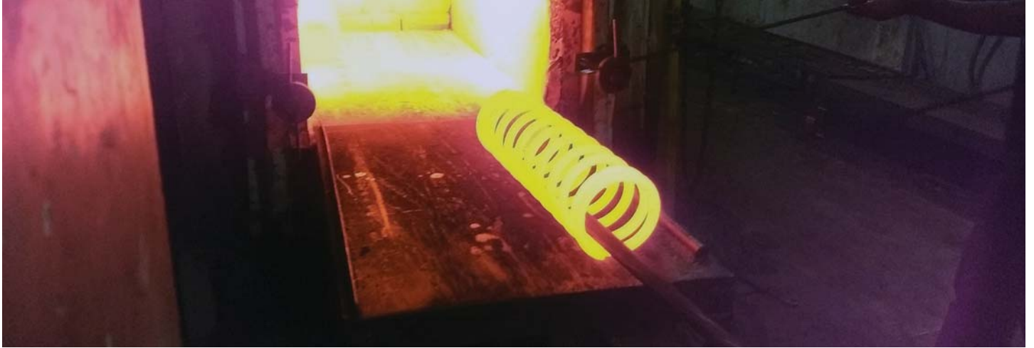
Heat Treatment of Coil Springs
