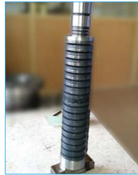
Disc Springs used in Tool Clamping
