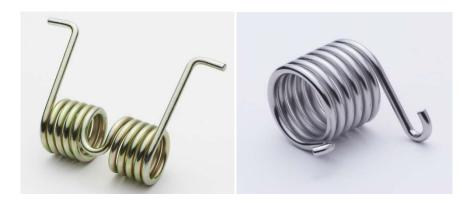
Torsion Springs resist external torque with angularly deflecting ends. Contrary to its name, the wire is subjected to bending stress and not Torsional stress. These are close wound springs. After deflection, the body length increases and coil diameter reduces.
