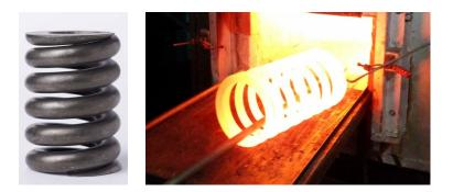
Hot-coiled springs are generally used in elevated temperatures, high load applications or in a corrosive environment. The transportation industry, Agriculture equipments manufacturers, and construction equipments manufacturers are some of the largest users of the hot coiled springs.
